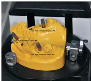
Figure 3c: Scan Posts on the Implant analogues
